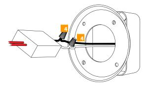
5 Connect red transformer wires to fixture wires, using wire nuts provided.
