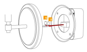
6 Install backplate cover on mounted backplate with hex nuts.
